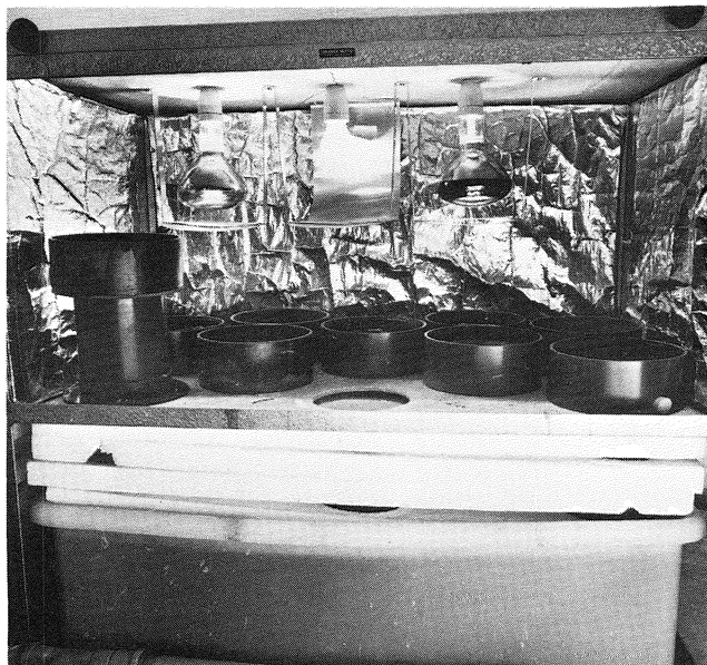
Fig. 4. Extractor including cooling unit (water bath and tubes). Front of extractor removed; eight containers immersed into the water bath, to the left container elevated by means of PVC-ring (N. Skyberg phot.).
